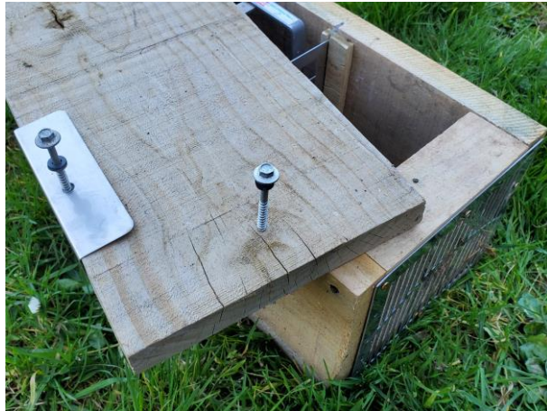
Photo 7 suggested position of third screw in lid lined up with the top bracket to exclude kea and guard against human error or screw failure.
